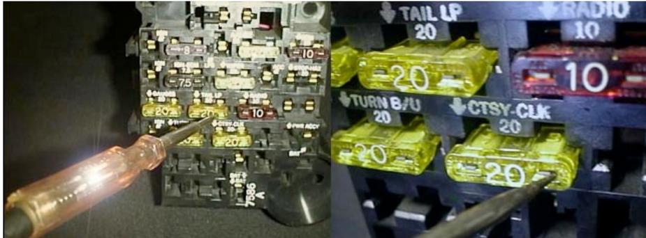
Remove the fuse and use the test light or voltmeter to verify which side of the fuse connection is “hot”. Either replace this fuse with an accessory fuse or place a fuse tap onto the removed fuse on the hot side fuse terminal.
