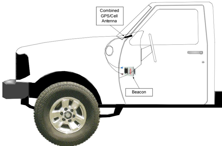
Orientation of the beacon is not critical to its performance but consideration should be given to visibility of the indicator LEDs. In some instances visibility is desirable and in other it is not. The LEDs do provide feedback about the operation of the beacon, so easy viewing is desirable for unconcealed
