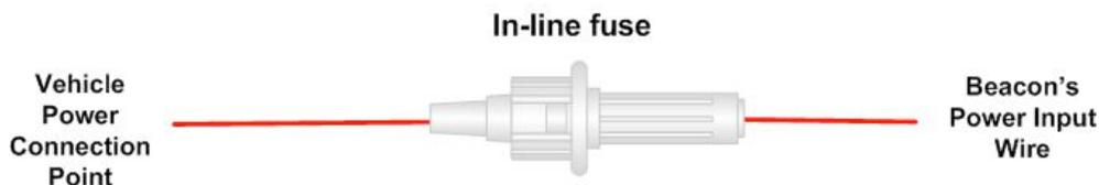
Install the fuse as close to the vehicle connection point as possible. This will allow the fuse to protect against short circuits in the beacon's wiring harness as well as within the beacon itself.
